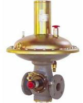
The series-MR pressure regulators are selfoperated and spring controlled, with single seat and counterbalanced shutter. All the types can be equipped with a built-in slam-shut valve which is operated by OS/66-R o OS/66-R-AP
